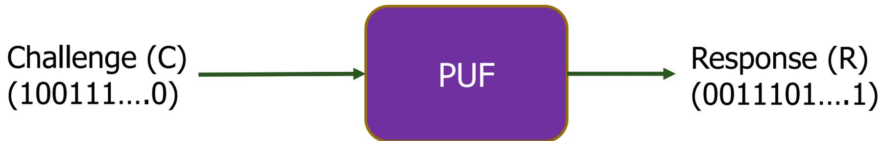
Only an authentic hardware can produce a correct Response for a Challenge.
