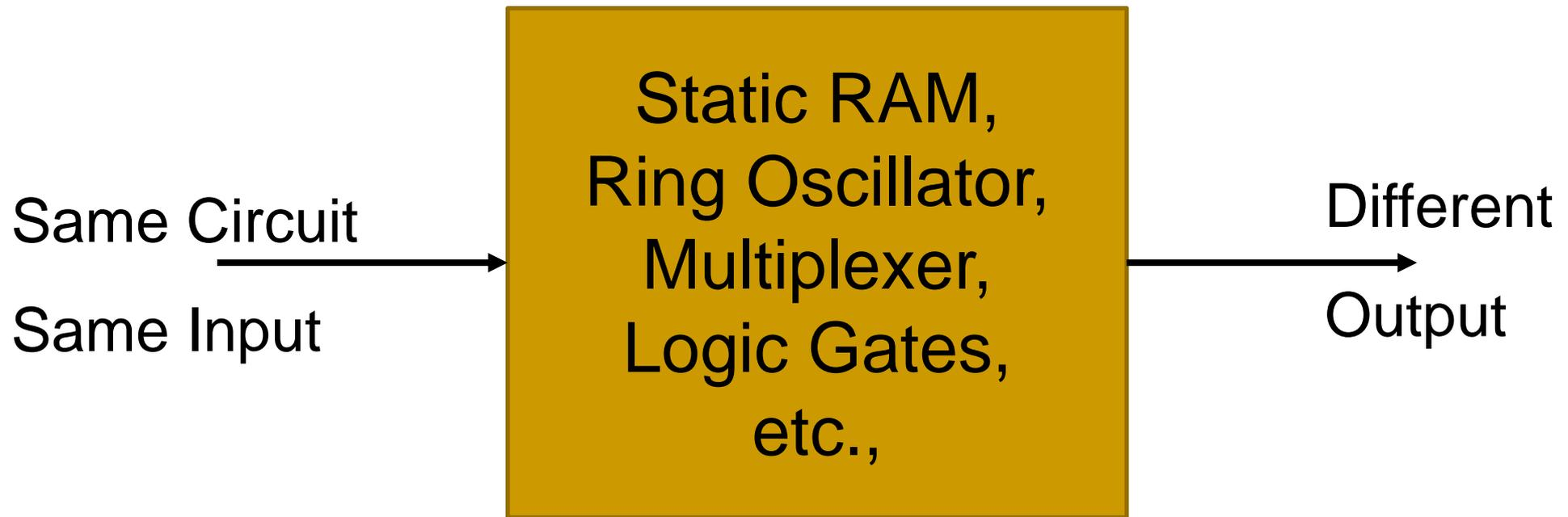
With the same circuit and the same input, we get different output due to process variations.
