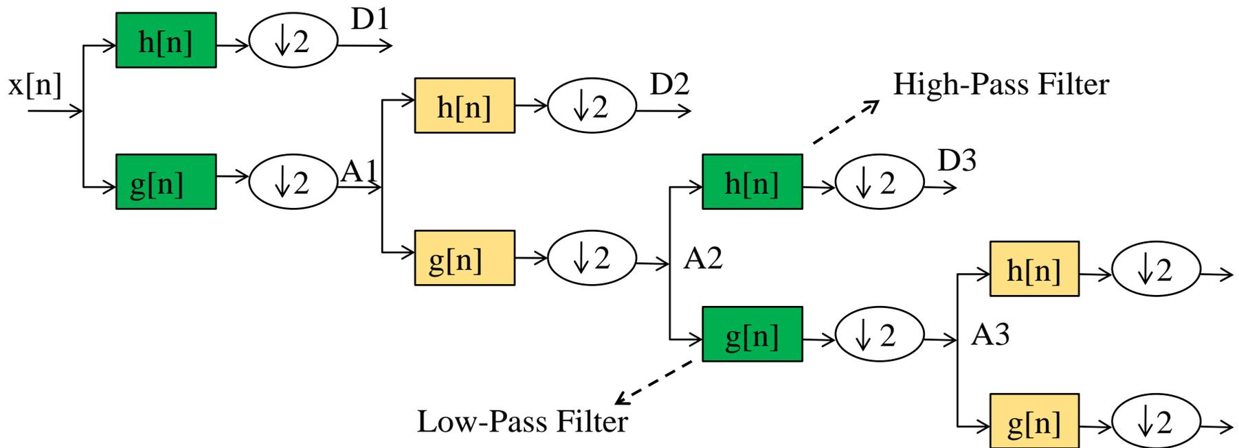
Fig. 7. Four level wavelet decomposition of EEG
