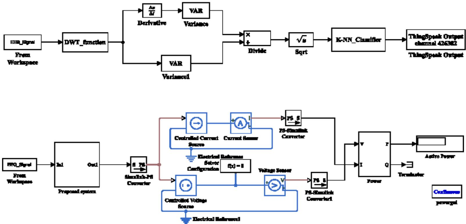
Fig. 9. Simulink Implementation (Top) System (Bottom) Power measurement set up
