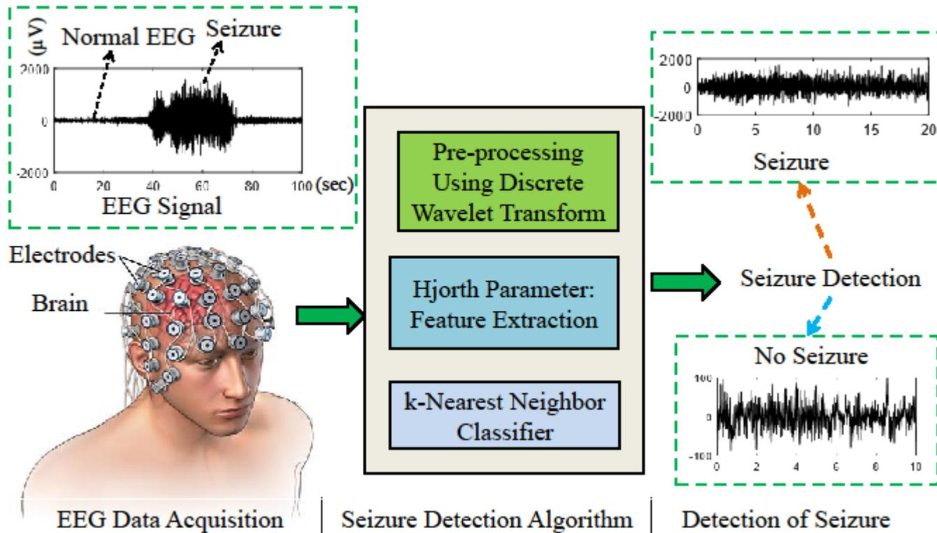
Fig. 2. A schematic overview for the proposed seizure detection paradigm
