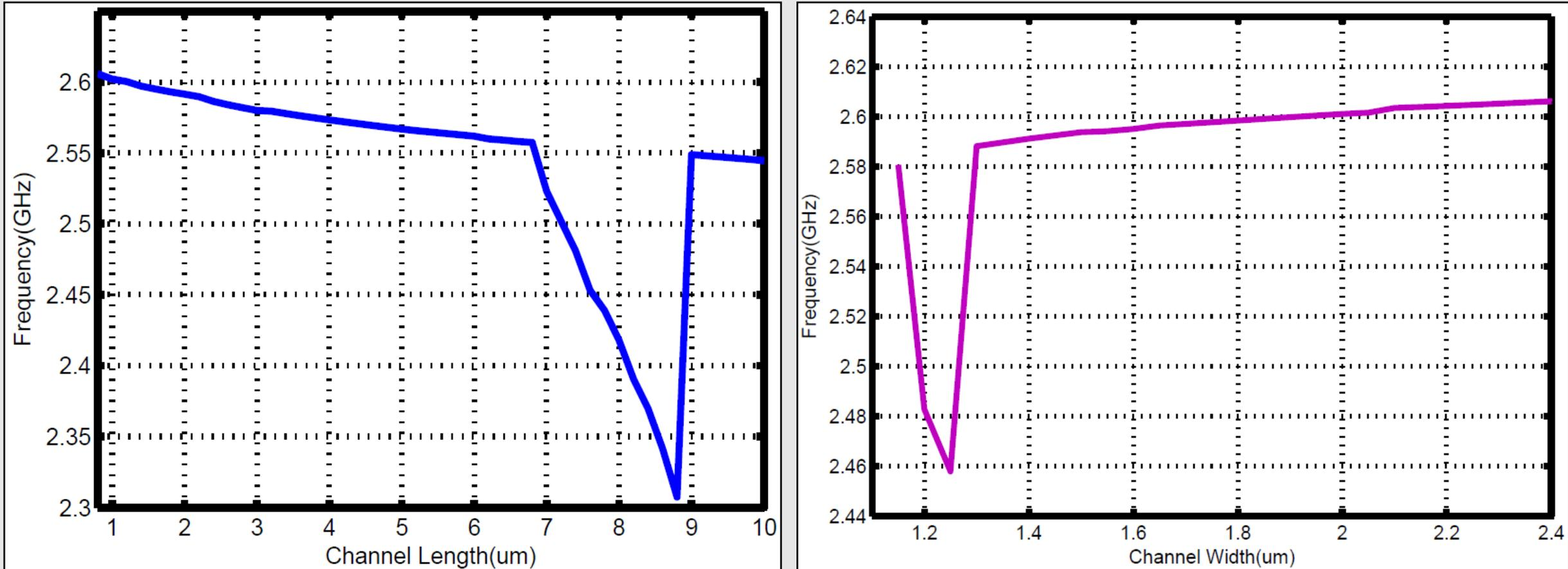
Fig. 6. Frequency of the GFET based LC-VCO vs Channel length and Channel width
