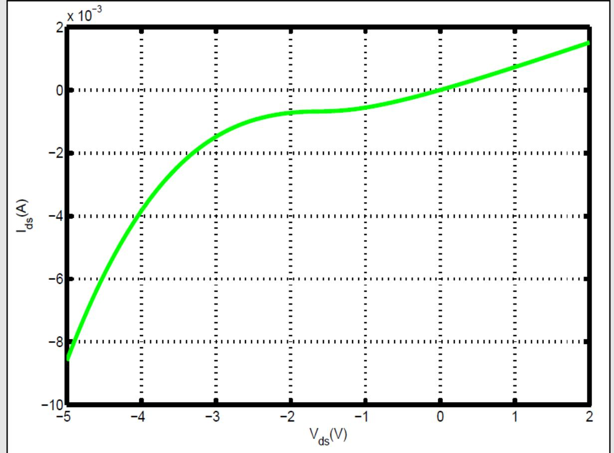
Fig. 2. I-V Curve of N-type and P-type GFET around operating region
