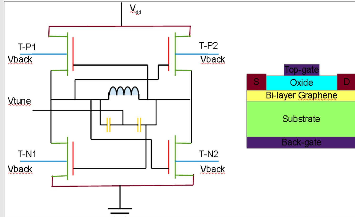
Fig. 1. GFET based LC-VCO with GFET-2D cross-section (left)
