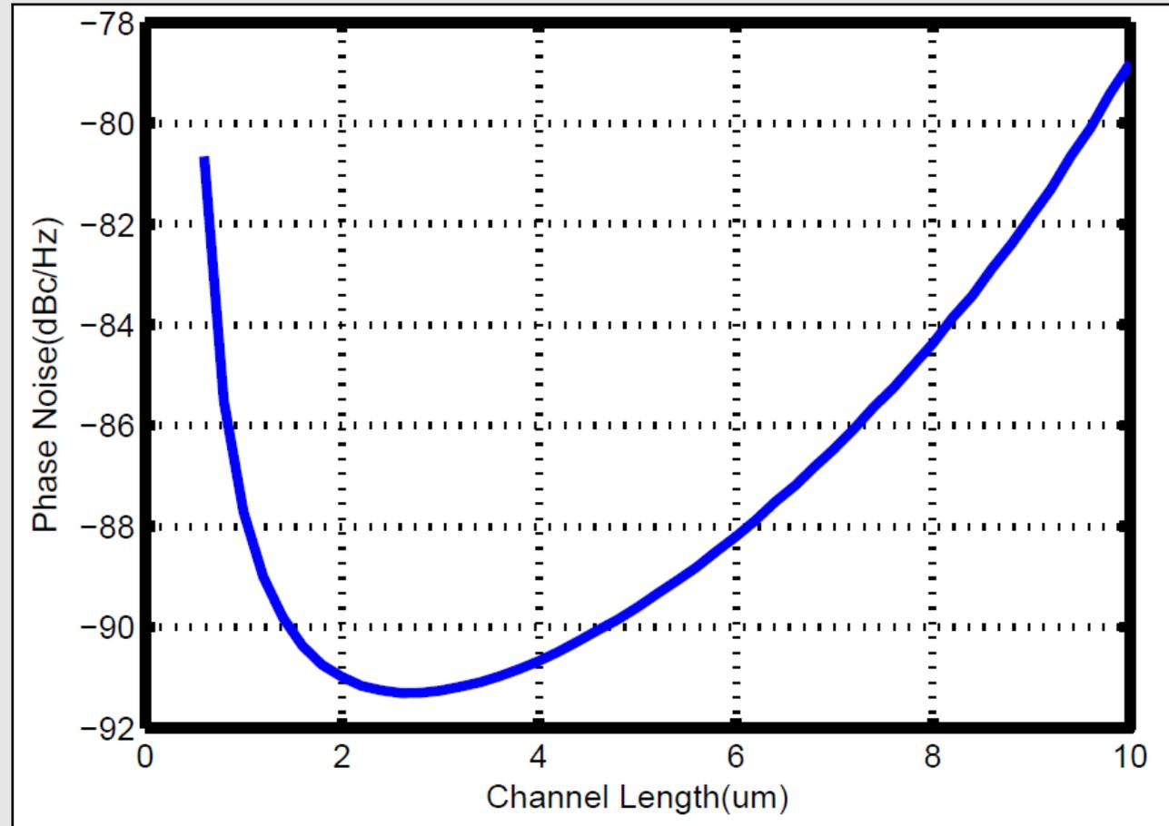
Fig. 8. Phase Noise of the GFET based LC-VCO vs Channel length and Channel width
