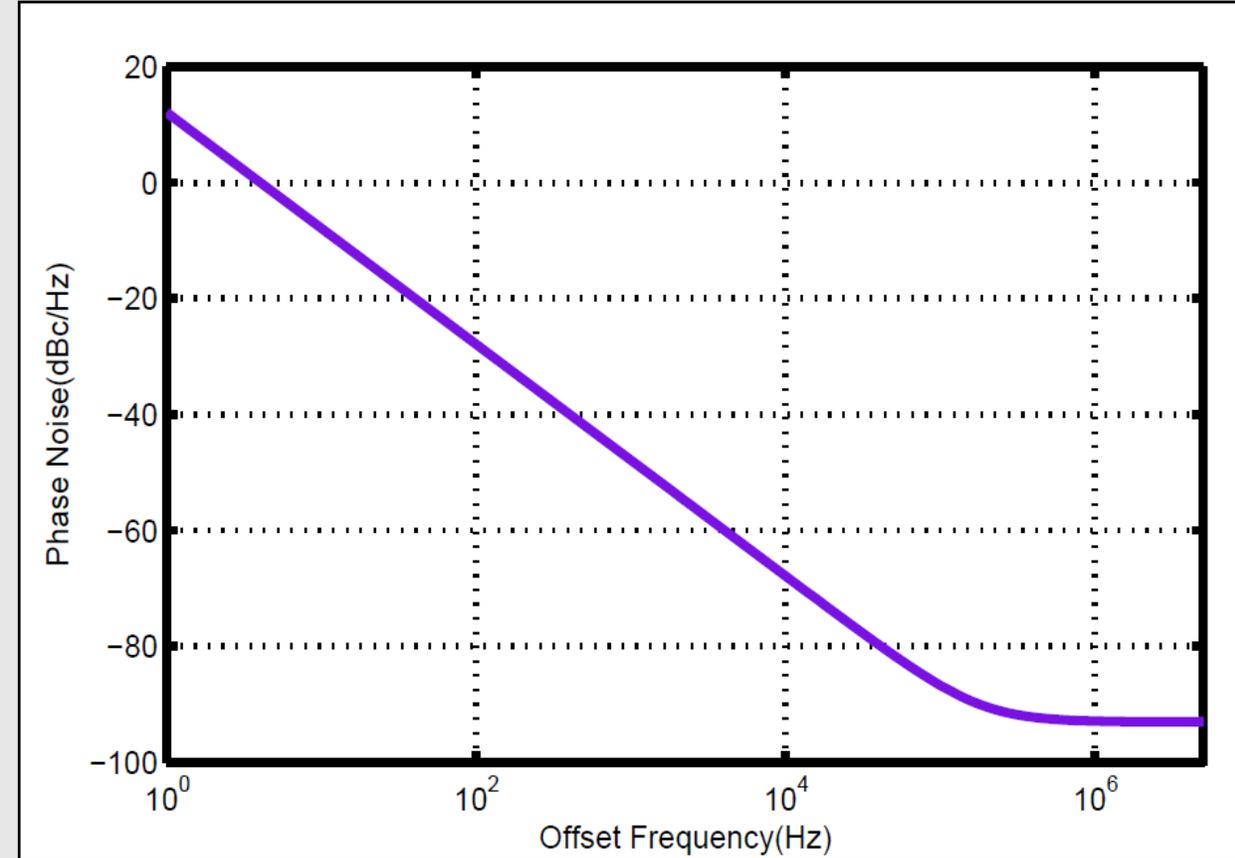
Fig. 9. Tuning Range and Phase Noise of Optimized GFET based LC-VCO
