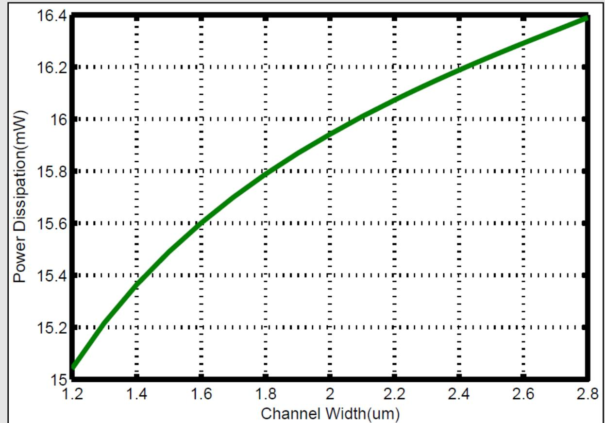
Fig. 7. Power Dissipation of the GFET based LC-VCO vs Channel length and Channel width
