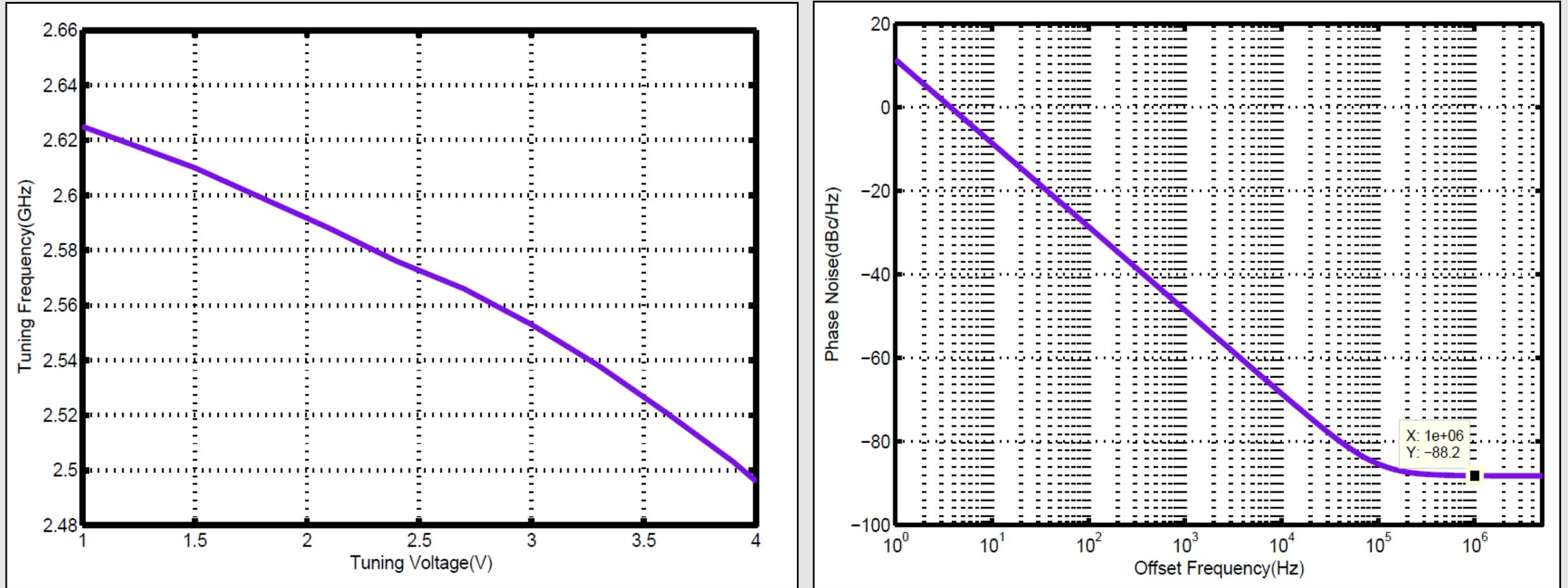
Fig. 3. Tuning range and Phase noise Characteristics of the baseline GFET based LC-VCO
