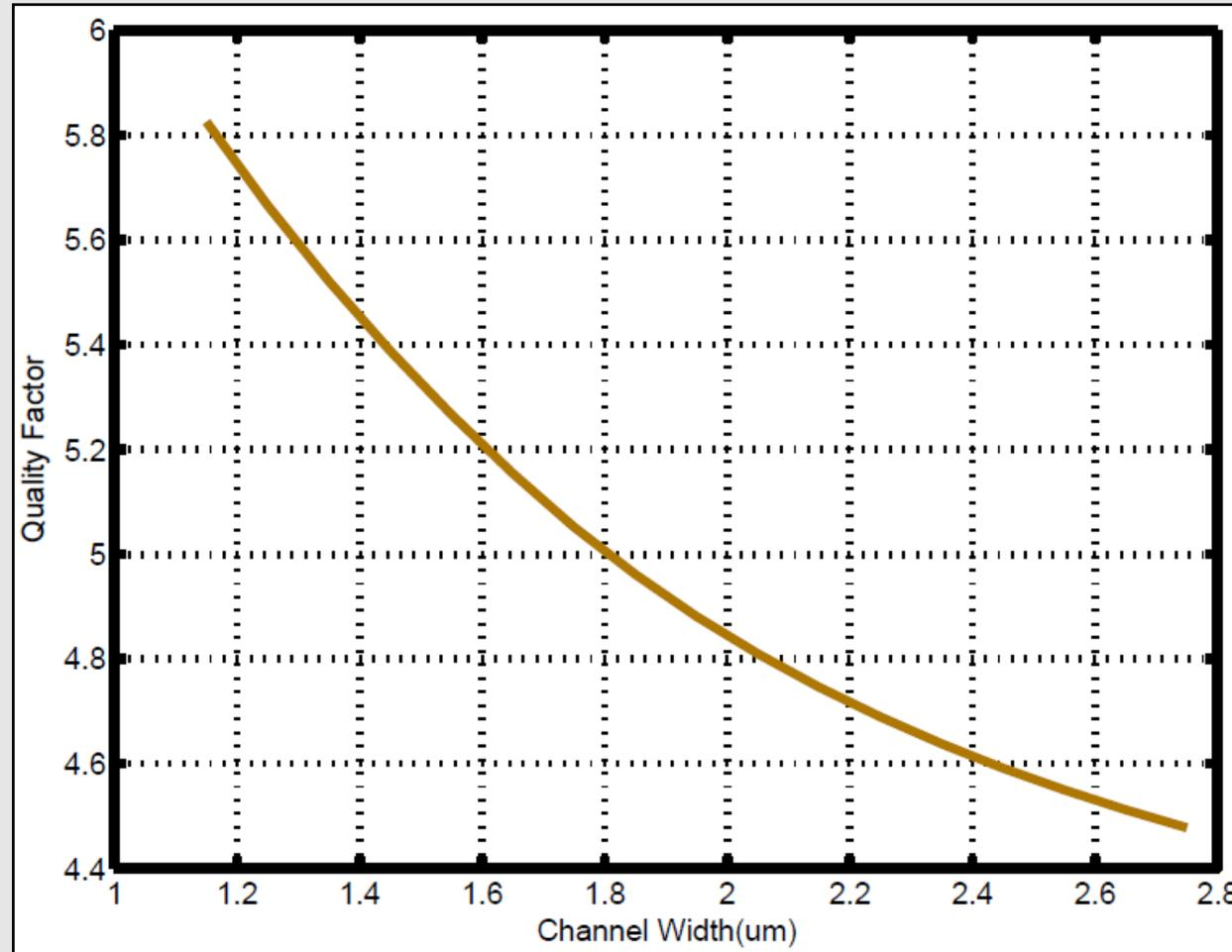
Fig. 5. Quality Factor of the GFET based LC-VCO
