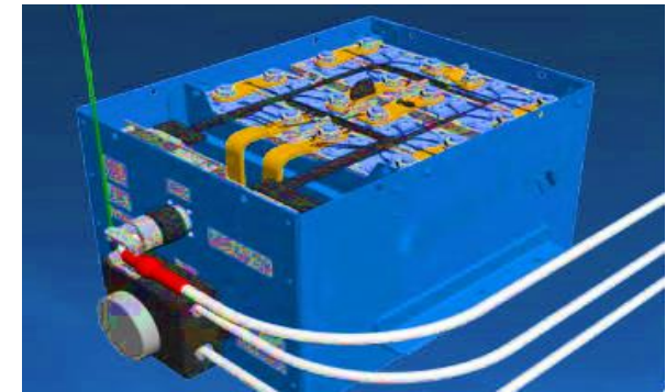
One 787 Battery: 12 Cells / 32 V DC
