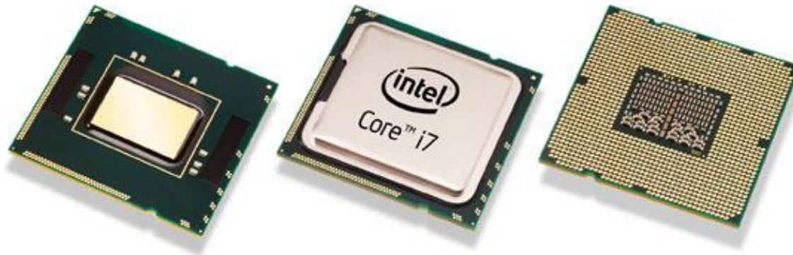
Intel Core i7 LGA1366 processor has 1366 pins.
