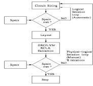
The proposed methodology performs the multiple (X) iterations automatically on a parasitic parameterized netlist derived from the layout. The manual iteration is reduced to 1. To have a process variation robust design, process variation analysis is introduced in the design flow.
